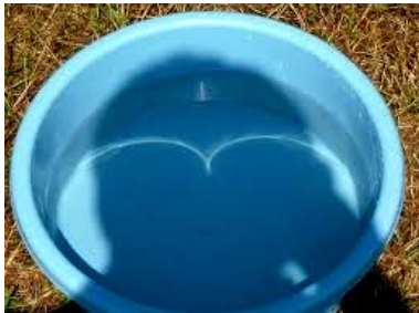
Fig. 1. Caustic as a manifestation of spherical aberration of spherical or cylindrical concave mirror: (a) geometrical and (b) physical counterpart of the caustic [7]
