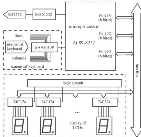
Fig. 2. Simplified electronic diagram of basic module
