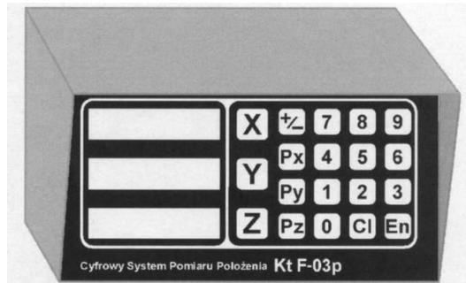
Fig. 6. Tri-axial digital system of position measurements
