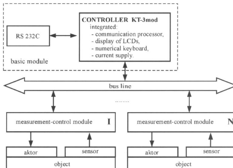
Fig. 1. Block diagram of the digital system of the position measurement
