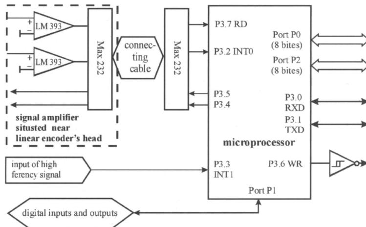
Fig. 3. Simplified electronic diagram of measurement-control module with attached capacitive linear encoder
