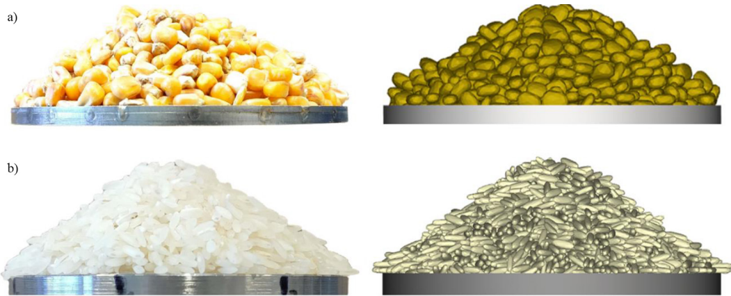
Fig. 4. The pile formation in the calibration of simulation parameters by static angle of repose (left – physical experiment, right – DEM simulation)
