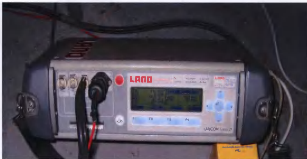
Rys.5.4. Analizator spalin Lancom II firmy LAND Instruments International
