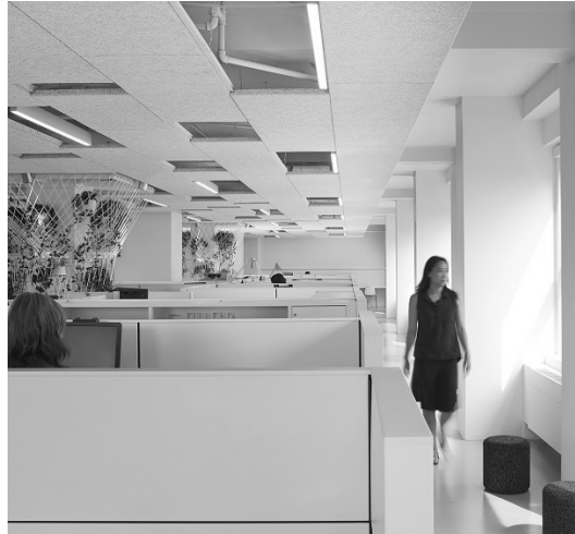
Fig. 1. Location of row of individual box workstations in a distance from external glazed facade in order to reduce direct solar thermal gains and assure equal natural lighting at workplaces in an open space office. NRDC, Chicago, USA, 2013, proj. Studio-Gang Architects (fot. S. Hall), Hedrich Blessing, certificate LEED-CI level Platinum. (source: http://www.nrdc.org/cities/building/chioffic.asp , http://www.earchitecture.co.uk/chicago/natural-resources-defence-council-office (access: 12.08.2015))
